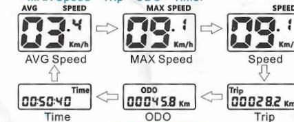
Note: If there is no operation for 5 seconds, the meter will return Speed (Real-Time) display automatically.
